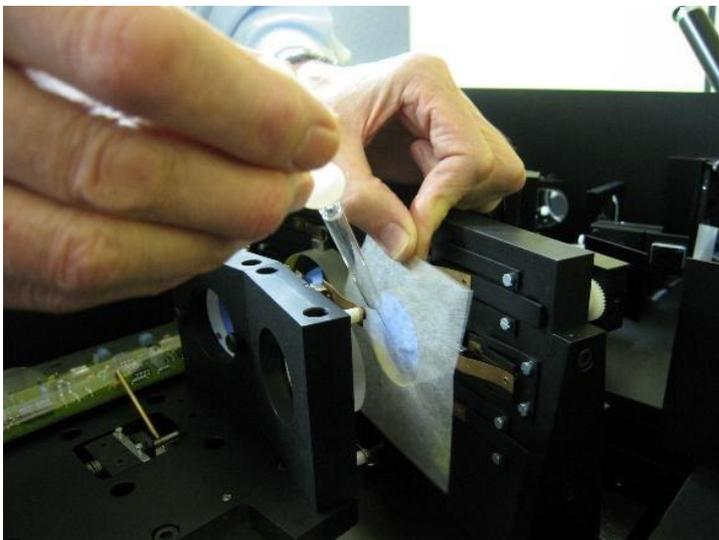
Apply clean alcohol or acetone via a fine pipette to a lens tissue held as low as possible and touching the mirror. The fluid should wet the tissue so that it adheres to the whole mirror area. No excess fluid should be allowed to drip down.
