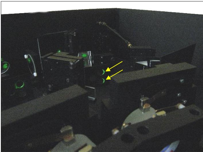
With full alignment, remove the piece of card so that the transmitted beam reaches the prism PR1. Look on the small aperture after FP2 and you will probably see some light striking the sides of the first two holes as shown here. The prism can be rotated slightly about a vertical axis until these multiple reflections disappear.
