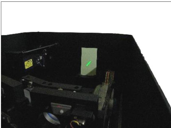
Place a piece of card in front of M3 and observe the light transmitted by FP1. Probably 1 fringe will be visible. If no fringe is visible, adjust Z until a fringe comes into view.
