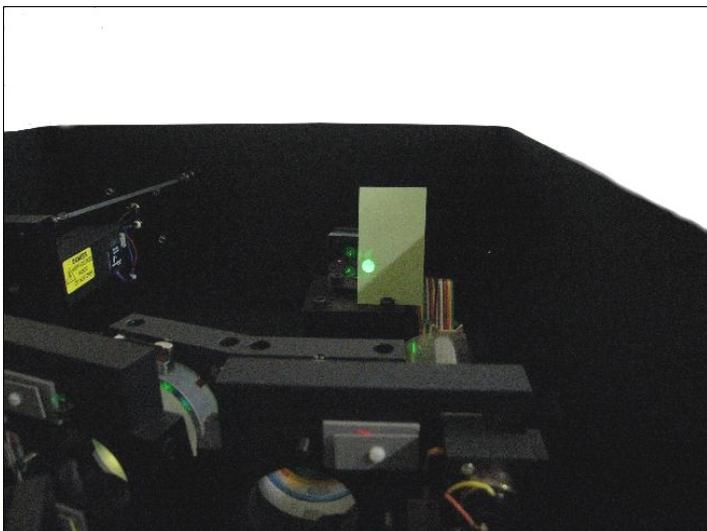
If you have done a good job of alignment you should now see the transmitted light in front of the cat's-eye M4. Tweak the alignment piezos to give maximum intensity.
