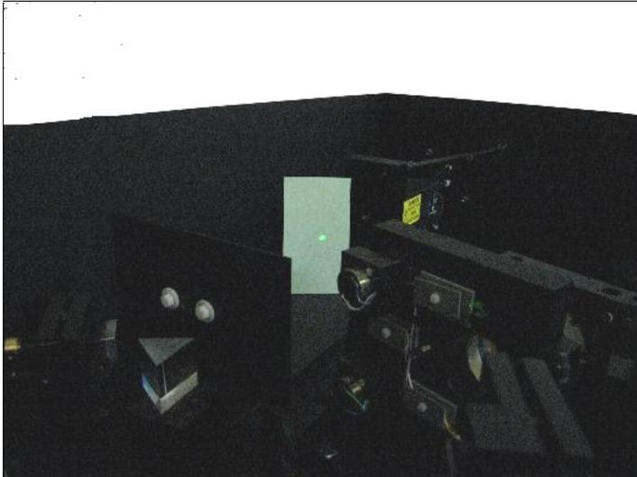
Check the beam after lens L2. The beam should be circular in section and not clipped. If clipped, try rotating the glass block G2 to obtain a better transmission. (G2 can be rotated about its vertical axis by applying a light force).
