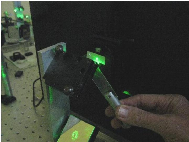
If you are using back scattered light, hold a thin glass plate in the scattered beam close to the input pinhole, and rotate it slightly so that the light reflected from FP1 falls onto a small piece of paper placed near the pinhole.
