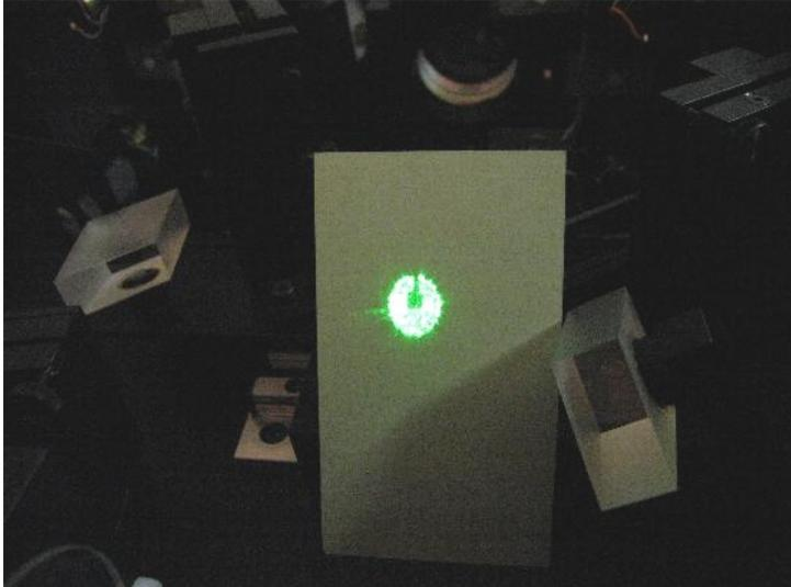
The next step is to make sure that the light falling on FP1 is reflected back out of the input pinhole. Choose the 1000m pinhole and set the optics to "Tandem".
