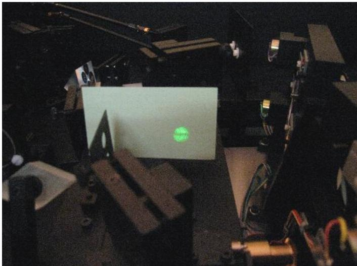
Check the alignment mode optics by switching to “align”. Place a piece of card in front of BS2 as shown, and the light reflected from FP1 will be seen. When FP1 transmits, the reflection will go dark. Typically a dark fringe will be seen which can be adjusted to fill the field of view using X1, Y1 and Z.
