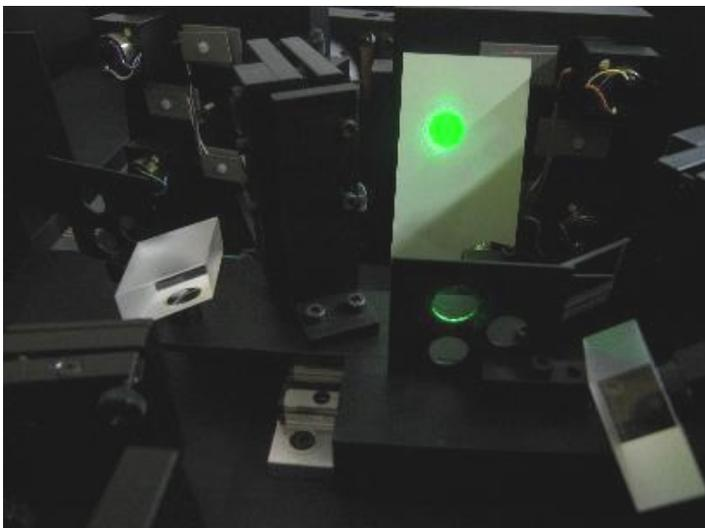
Check that a nice uniform wavefront is seen inside the spectrometer.
